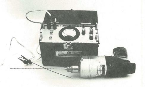
The Shigometer for detecting discolored wood and decayed wood in living trees and utility poles consists of a portable battery-operated drill with a long narrow drill bit, a twisted-wire probe that is inserted into the hole made by the drill bit, and a meter that produces a pulsed electric current and measures resistance to 500 K ohms. When the probe tip passes from sound to unsound tissues an abrupt decrease in resistance is indicated on the meter.
