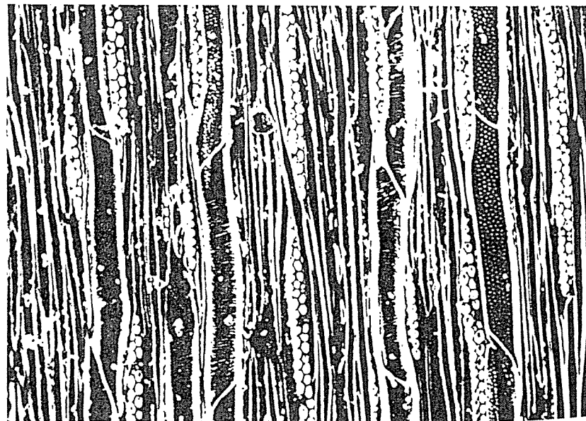
FIGURE 4. A 100× scanning microscope view of a tangential section of normal red maple sapwood
