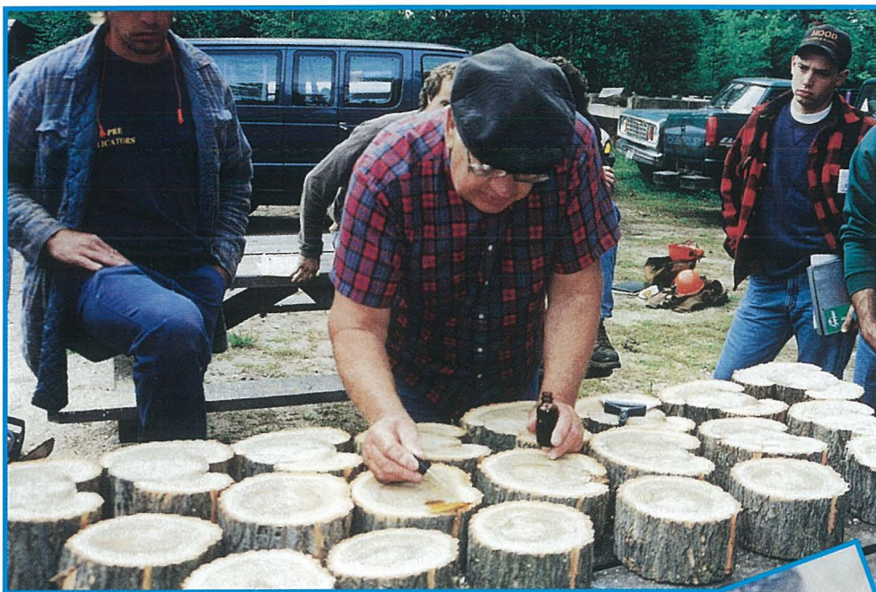
Dr. Alex Shigo demonstrates the IKI staining method.
