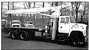
1993 Ford LNT8000. 8.3 Cummins 9 sp, 100,000 miles with 17-ton R.O. crane. 128' hook height. $76,500
